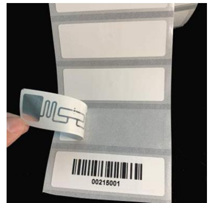
A “smart label” that includes an RFID inlay and a barcode can provide interoperability across available technologies.
